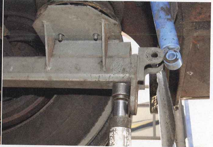
3. The lower shock mount bolt is loosened, but before it is removed, the rear of the trailing arm is supported to prevent it from falling down.
