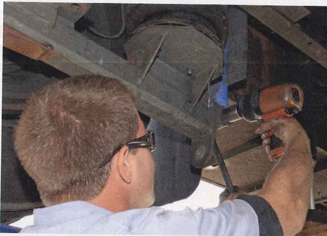
3. The lower shock mount bolt is loosened, but before it is removed, the rear of the trailing arm is supported to prevent it from falling down.
